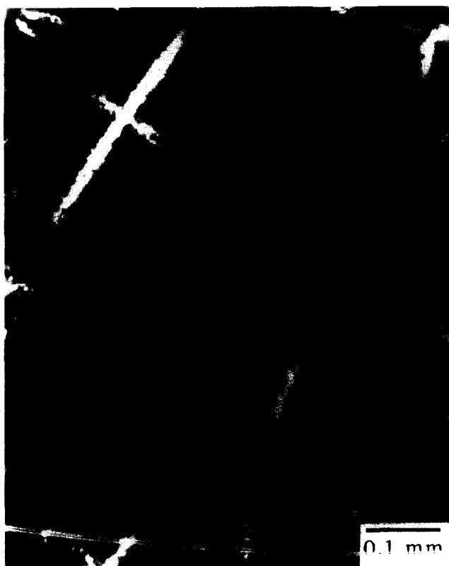
Figure 6 Optical micrograph (crossed polars) of a P(mOBA)/ONA sample polymerized at 197°C for 23 h
